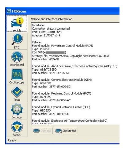
Here is a screen shot and the tools you can use BUT remember to back up the module you are tinkering with on to your hard drive so if you do something wrong you can re-install the original parameters. You do not want to be in deep do-do!
