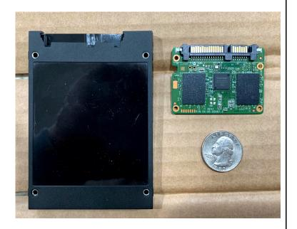
Here is a Sandisk (I removed the label) to see how it came apart. It has no screws but snaps together. Yes, the printed circuit board is less than half size. In fact, if you have a SD card that you use in your camera, it's smaller than the package. If you ever saw those micro chips that insert in a SD Card, it is small!!
