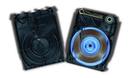
The 8 track cartridge opens to two half shells.
